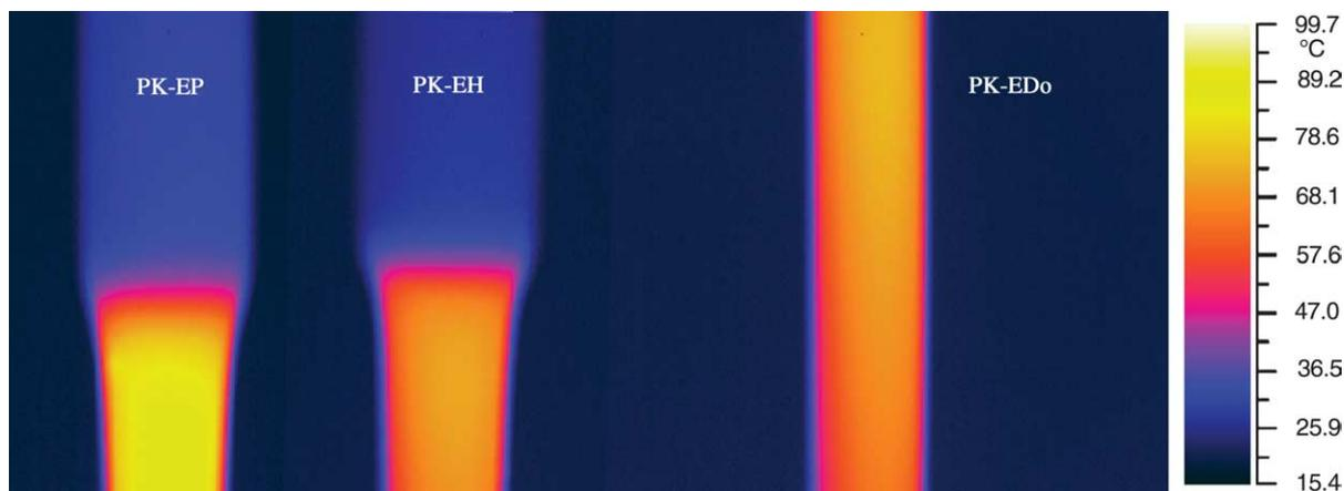
Fig. 12. Neck profiles for different polyketone terpolymers, PK-EP; PK-EH and PK-Edo; ambient temperature 20 °C, strainrate  $1.25 \times 10^{-3} \text{ s}^{-1}$ , (test speed 60 mm/min).
